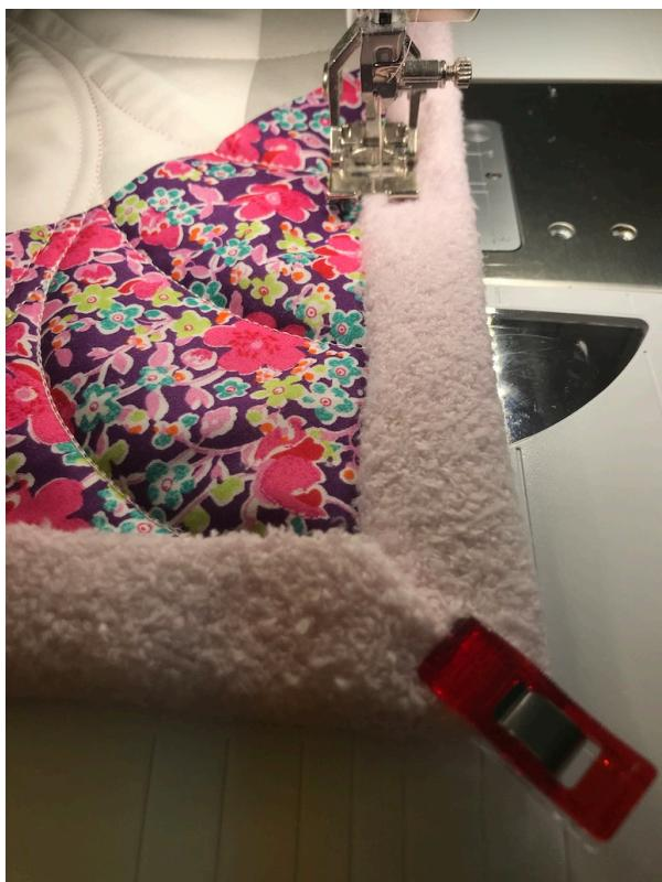
As I sew up to the corner I continue sewing until I have caught the folded piece of binding. With the needle still down, I pivot and sew out toward the corner.
