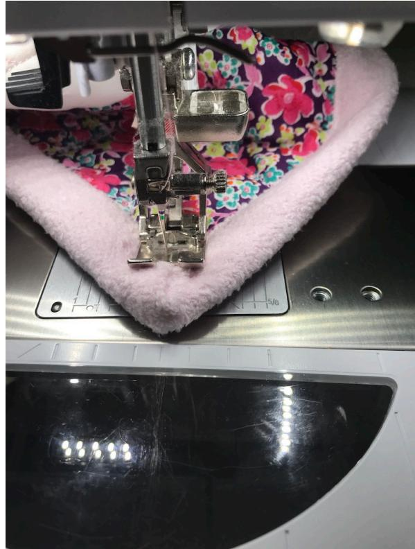
Once you reach the corner, reverse and sew back to the point where you pivoted. Keep the needle down and pivot so that you can continue with the next side.
